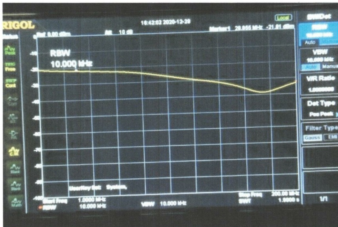
Figure 1: My kit attenuator swept from 1MHz to 200MHz and set to 20dB attenuation. The vertical axis is in 10dB increments, the second horizontal line from the top representing 20dB of attenuation.
