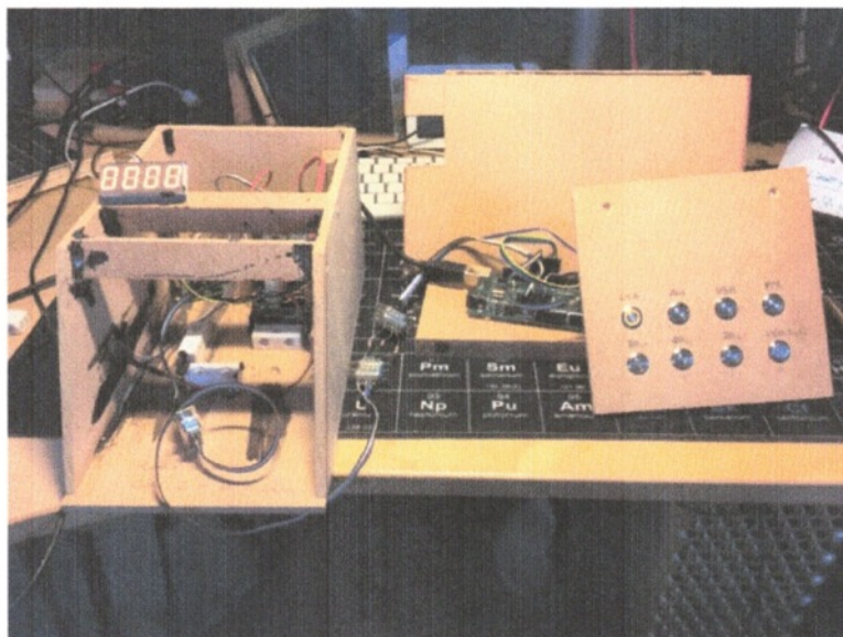
Late 2018 Proof of Concept - (Pro mini micro-controller & “MDF enclosure”): 8 buttons : 4 for Mode change, 4 for Band change.
