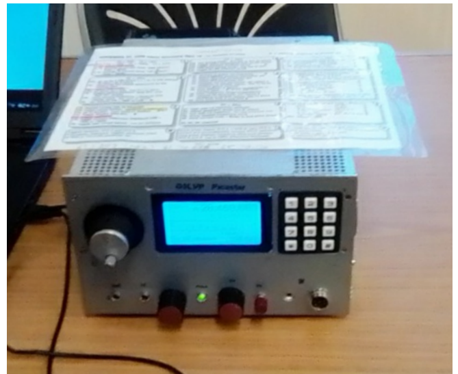
Homebrew Software Defined Radio (SDR) by Ken G3LP
