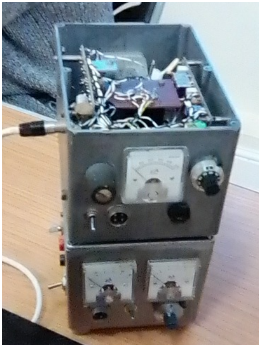
10GHz wideband FM transceivers by G4CIB
