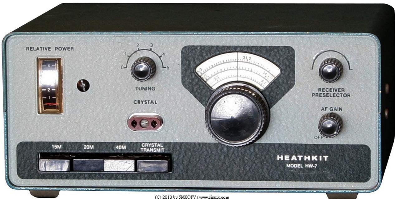
In the meantime I had built my HW7 which was a compact 2 watt CW direct conversion transceiver covering 80m, 40m, 20m and 15m. I eagerly awaited the issue of my call sign which duly arrived on 11<sup>th</sup> July 1973. Now, here's a strange thing – the first entry in my log for an HF qso using G4CIB is
