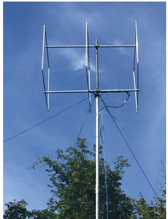
Arron M0HNNH's 3 element 70MHz Quad antenna
