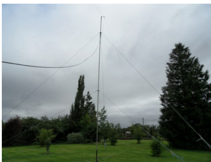
The Antenna Inverted V dipole fed with 300 ohm cable with an 11m pole in the centre.
